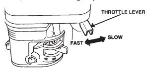
Figure 30. Throttle Lever
